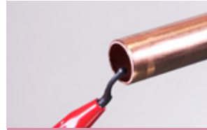
3. Use a pencil type deburrer on internal edges
